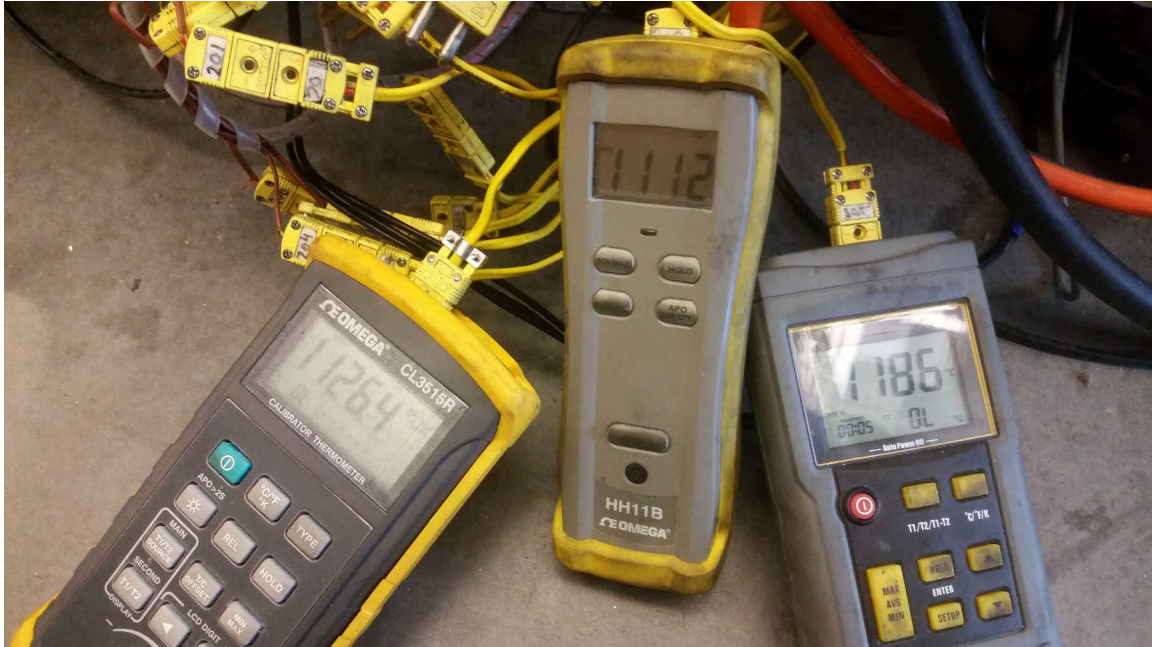
Figure 51: Backup monitoring/control system to circumvent signal interference issues
