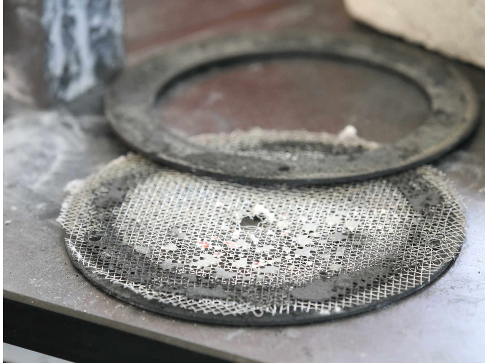
Figure 53: Tungsten mesh un-bonded from graphite mount after the reaction bond suffered severe oxidation
