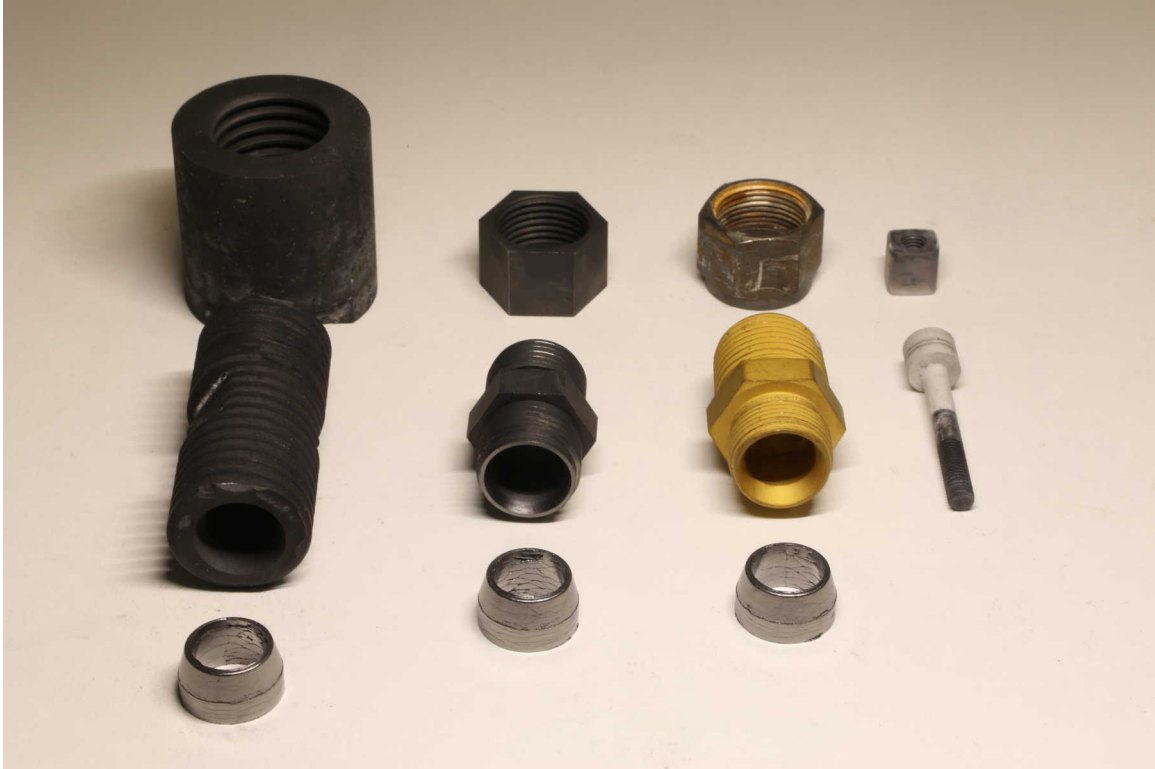
Figure 23: C union, W union, CrN coated steel union, and Shapal bolt for reference (from left to right). The C union is the largest because it has the lowest strength. Both the C and W unions are compatible with liquid Sn above 1350°C. The Shapal bolt, which failed, is shown as an example of the need to oversize brittle components.
