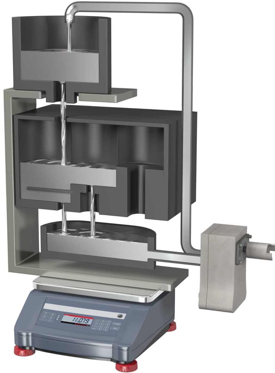
Figure 32: Calibration of the visual flow meter, experimental setup
