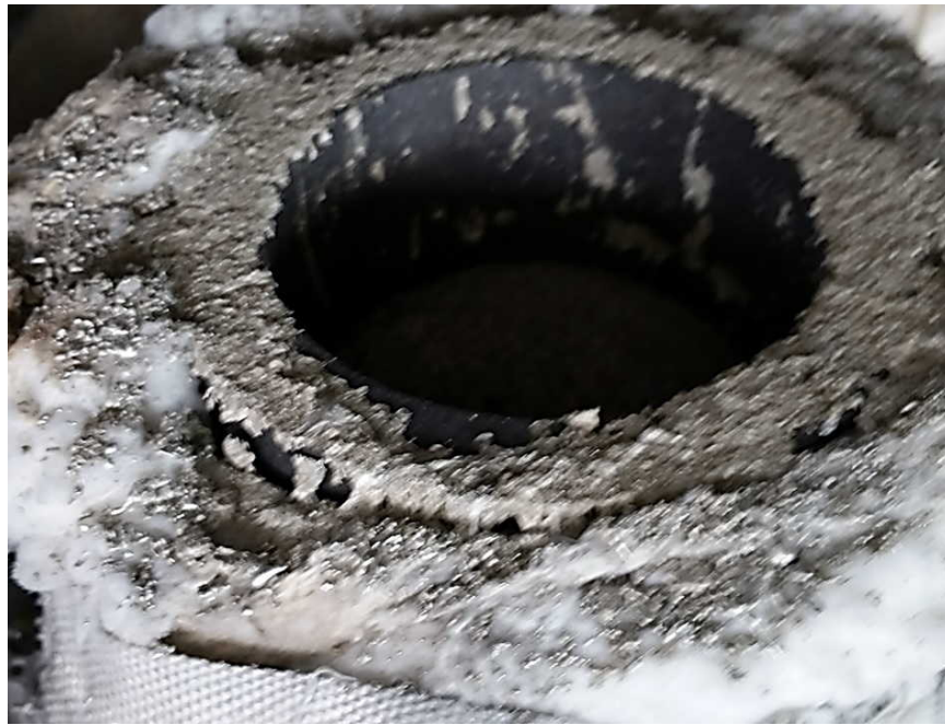
Figure 21: Splashed Sn around the reservoir from freefalling Sn inlet
