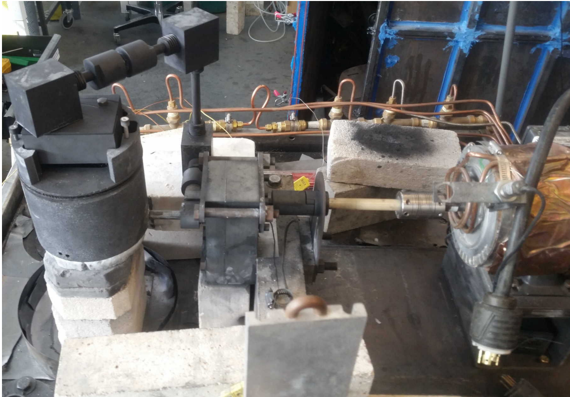
Figure 59: Pump system in configuration used for 72 hour test
