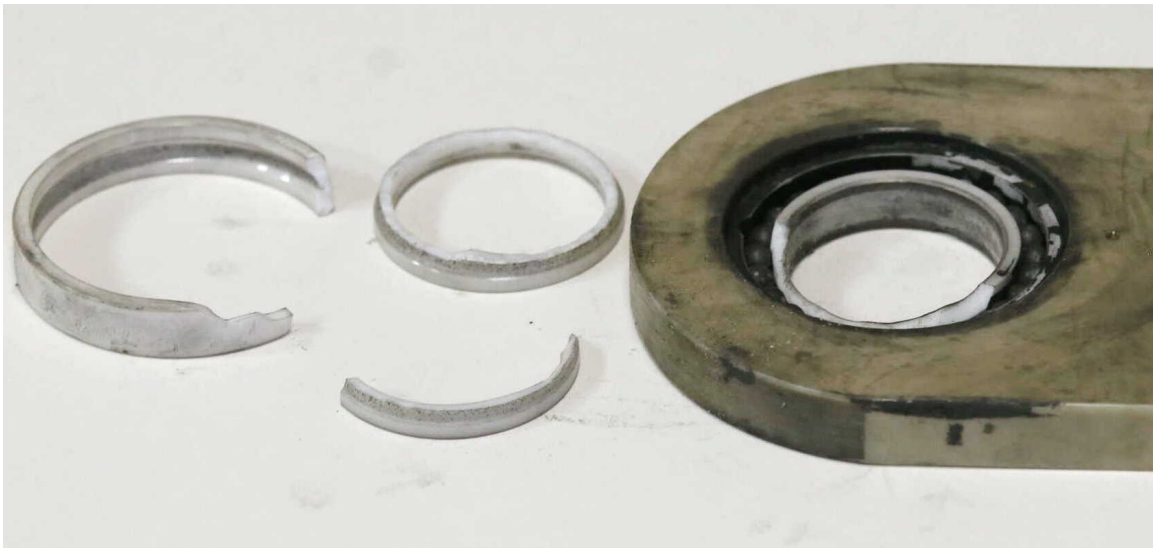
Figure 16: Zirconia ( ZrO_2 ) ball bearing failure
