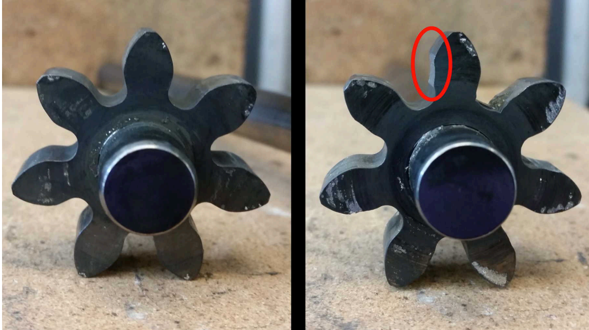
Figure 47: Corrosion on Inconel 625 gear teeth after scratching
