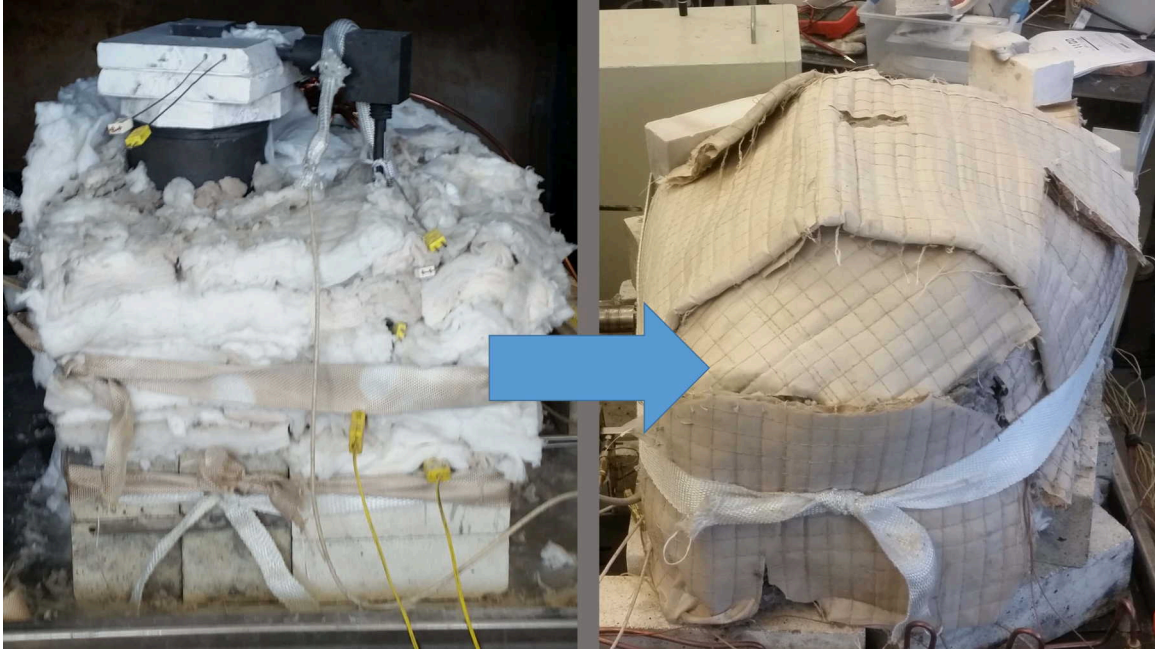
Figure 40: Insulation process for experiments above 1000°C
