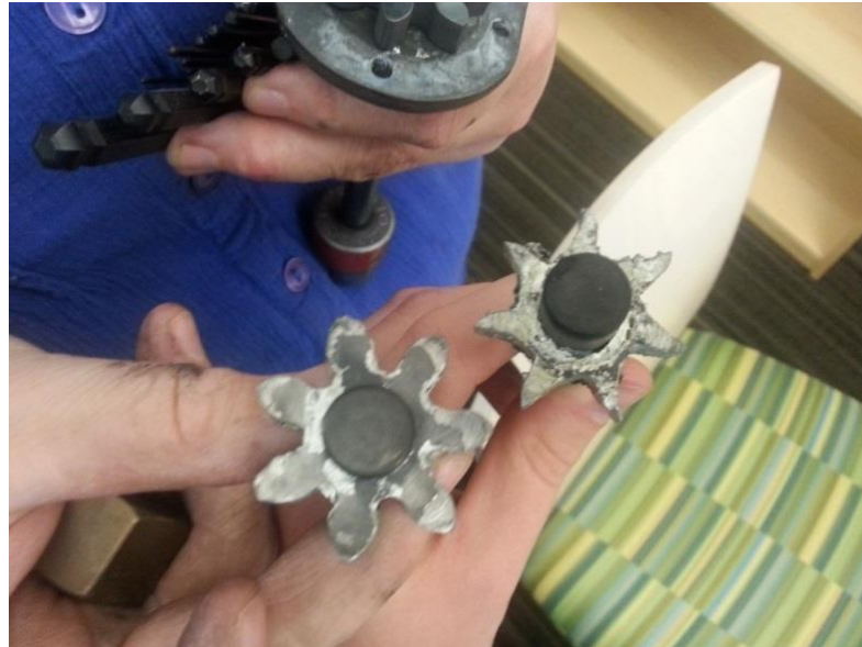
Figure 3: Relative corrosion of stainless-steel gears after less than 24 hours of contact with Sn at \sim 300^{\circ}\text{C} . the gear on the left was coated with CrN
