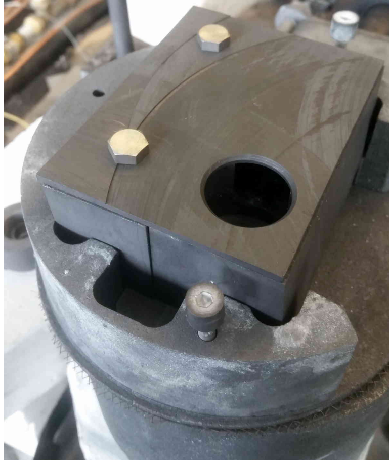
Figure 31: Visual flow meter with alignment pins and cover attached with W bolts
